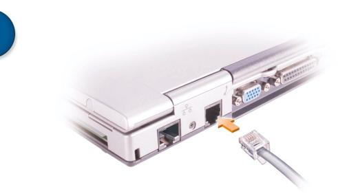
To use the modem, connect the telephone cable to the internal modem connector on the back of the computer.
